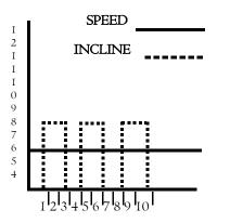
The **Fat Burn Program** is designed to vary the treadmill elevation, while maintaining a constant walking belt speed.
